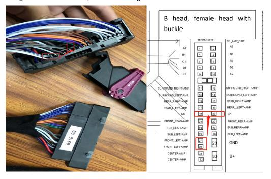
Method 2:Method 2: Change the position of the A plug, and use 2 wires to connect the PIN pin of the left front speaker of the original car and our 27.29 pin in parallel
